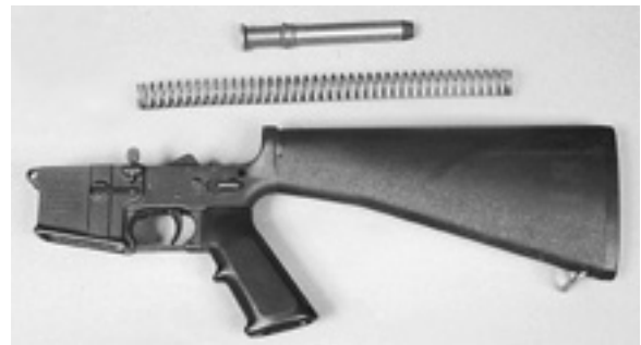
Figure 2-18. Lower Receiver Disassembled.
